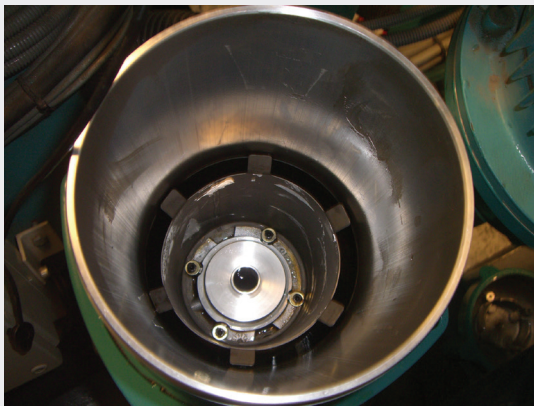
Same filter housing after cleaning. The AMSOIL flushing procedure removes contaminants from the gearbox before installing fresh oil. Peripheral components are cleaned manually.
